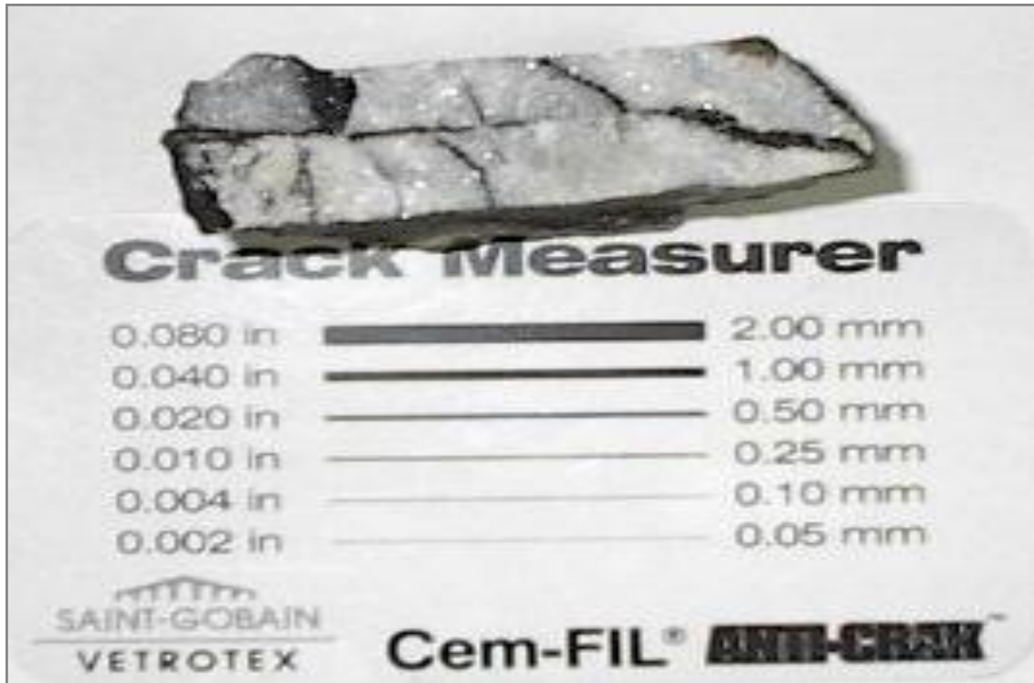
Figure 12: Sample of marble impregnated with Hot Bitumen
