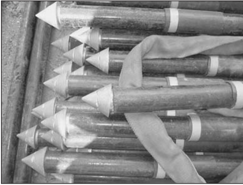
Figure 19. Sleeved grouting pipes with sacrificial cone
